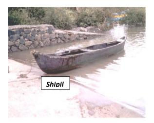
Mothi Shipil: Large hodi (boat). This type of boat is operated by 6-8 persons (preferably 8 persons). A typical boat is broadlyelliptic in shape, 12-12.5m long X4-4.5m wide. This boat is exclusively made of teak wood (Tectona
